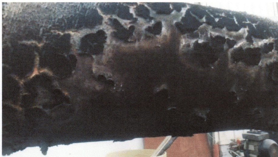
Picture no. 10: The test specimen after the fire endurance test. The exposed face of the pipe
